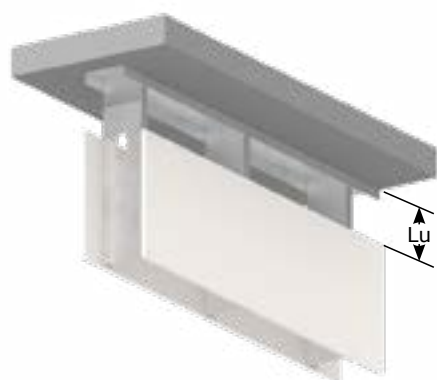
Non-Composite: Fully Braced Unbraced length is less than L_u
